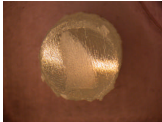
Figure 4. Stain on clear plastic due to solvent.
