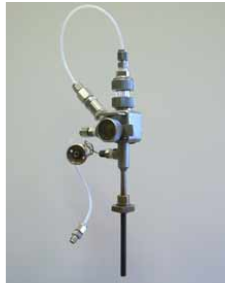
Figure 2. University of Connecticut thermal desorption device for GC/MS.
