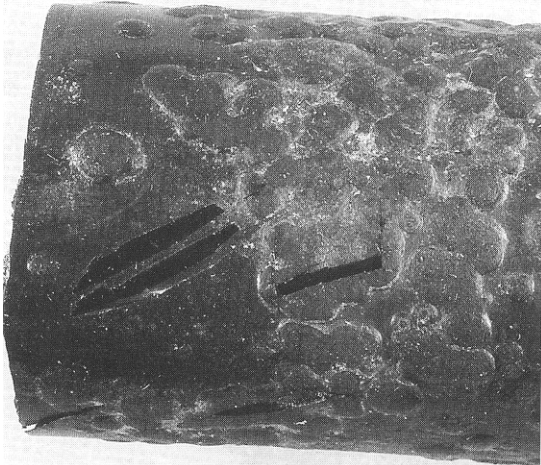
Figure 6. Neoprene rubber jacket blistered due to agricultural chemicals sprayed on it in a corn field where neoprene jacketed cable lay on the ground for a radar antenna (Ref. 1, p. 177, Fig. 6-17).
