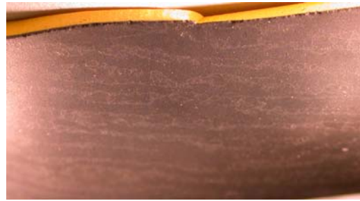
Figure 11: Image showing streaking down cuff.
