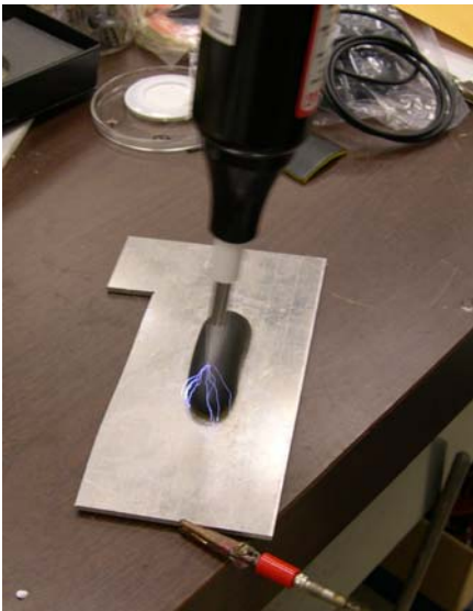
Figure 10: Inducing corona damage in the lab via tesla coil.
