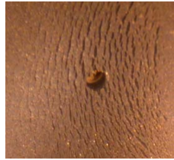
Figure 4: Optical microscopy image of "crazing" damage and perforation hole in black rubber outer surface.
